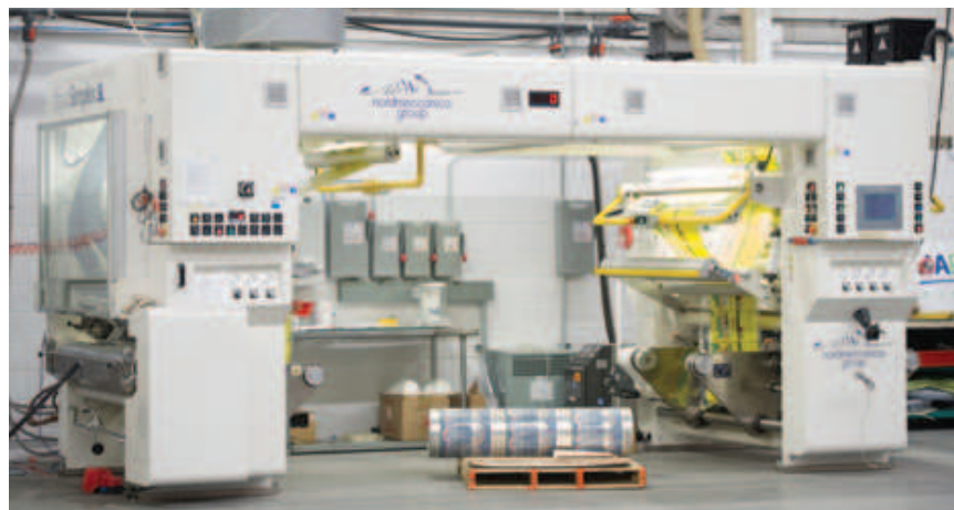
As part of its most recent major capital expenditure upgrades, Alpha Poly purchased a brand new Nordmeccanica Super Simplex SL two-ply solventless adhesive laminating machine.
