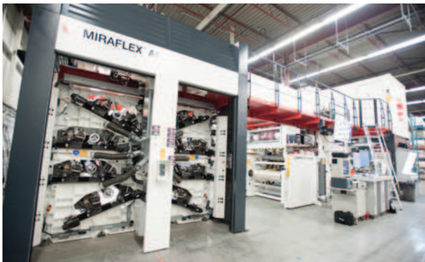
Manufactured by Windmoeller & Hoelscher, Alpha Poly’s new state-of-the-art Miraflex AM eight-color flexographic press was supplied by its Canadian distributor Webconverter Ltd.
