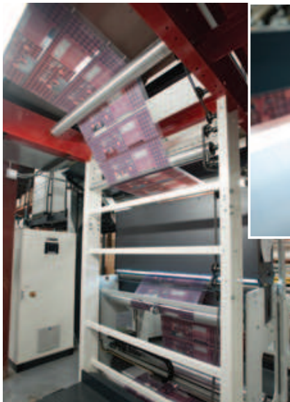
The cost-effective Miraflex AM flexographic press from W&H can accommodate print widths of 32 to 57 inches at speeds up to 1,300 feet per minute.
