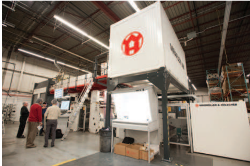
The eight-color Miraflex AM flexographic press has enabled Alpha Poly to increase its production speeds four-fold while presenting even higher quality graphics for customer products.
