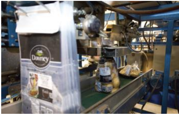
Working in line with a Volmpack 12000 six-head vertical filler, a Domino A-Series plus inkjet printer adds lot code data to closure tabs prior to placement onto polybags of potatoes.
